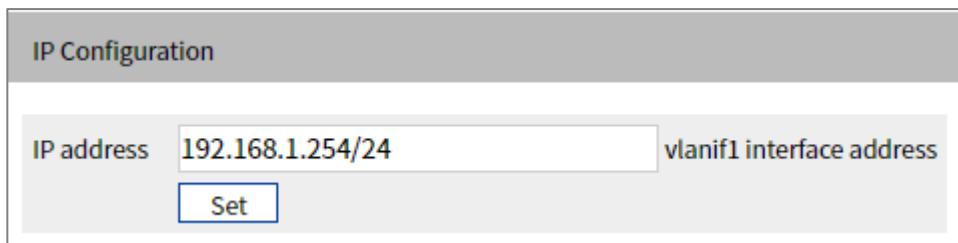
The screenshot shows a user interface for IP configuration. At the top, a grey bar contains the text "IP Configuration". Below this, there is a form with a light grey background. On the left, the text "IP address" is followed by a text input field containing "192.168.1.254/24". To the right of the input field, the text "vlanif1 interface address" is displayed. At the bottom of the form is a blue rectangular button labeled "Set".
