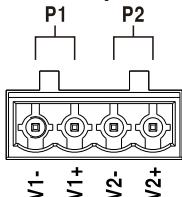
This device supports DC dual power input, P1 and P2 and provides 4-pin 5.08mm pitch terminal blocks. The power supply support anti-reverse connection. Power Supply P1 corresponds to power terminals V1 + and V1 -, and Power Supply P2 corresponds to power terminals V2 + and V2 -.
