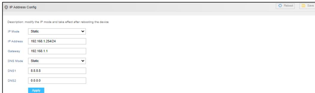
The screenshot shows the 'IP Address Config' interface. At the top, there are 'Reboot' and 'Save' buttons. Below that is a description: 'Description: modify the IP mode and take effect after rebooting the device'. The configuration fields are as follows:
