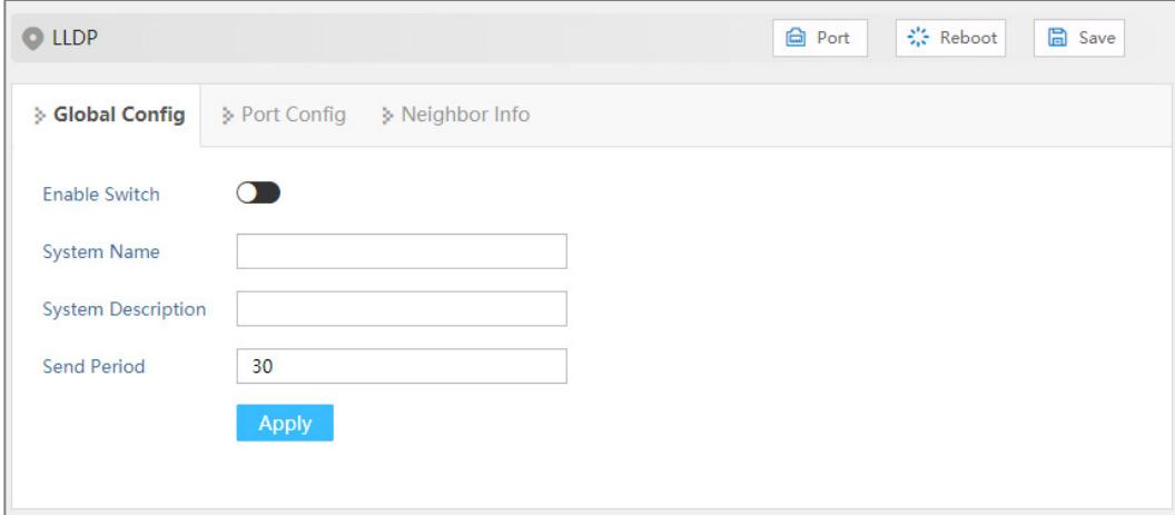
The screenshot shows the 'Global Config' tab of the LLDP configuration interface. It includes fields for 'Enable Switch' (checked), 'System Name', 'System Description', and 'Send Period' (set to 30). There are also 'Port', 'Reboot', and 'Save' buttons, as well as an 'Apply' button.
