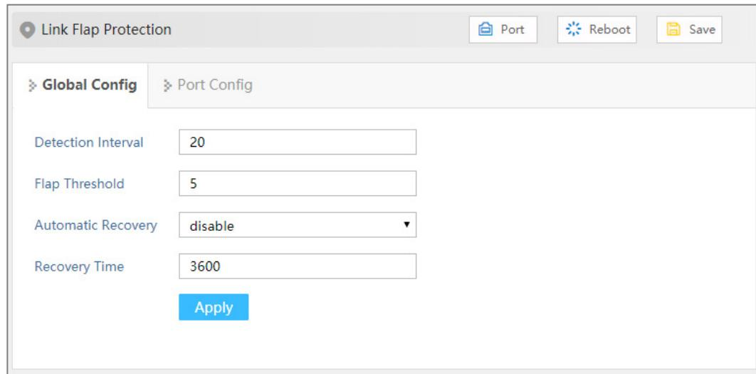
The screenshot shows the "Link Flap Protection" configuration interface. At the top, there are three buttons: "Port", "Reboot", and "Save". Below these are two tabs: "Global Config" (selected) and "Port Config". The "Global Config" tab contains the following configuration fields:
