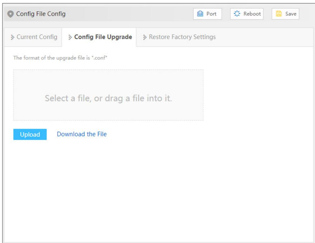
The main element configuration description of configuration file upgrade interface:
