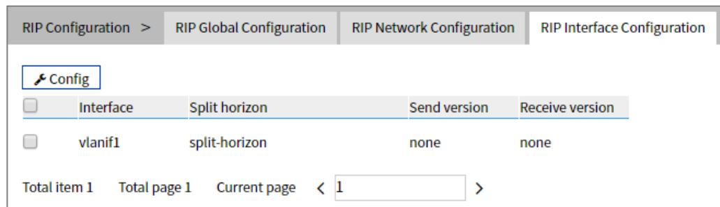
The main element configuration description of interface configuration interface:
