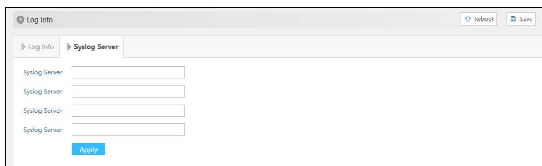
The screenshot shows a user interface for configuring a Syslog server. At the top, there are two tabs: 'Log Info' (which is the active tab, indicated by a blue border) and 'Syslog Server'. Below the tabs, there are four input fields, each labeled 'Syslog Server' and containing a placeholder IP address. At the bottom of the interface is a blue 'Apply' button. In the top right corner, there are two buttons: 'Reboot' and 'Save'.
