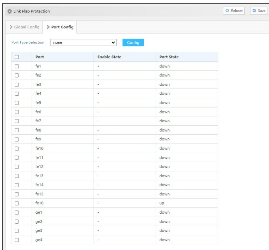
The screenshot shows a configuration interface for Link Flap Protection. At the top, there are buttons for 'Reboot' and 'Save'. Below that, a navigation bar has 'Global Config' and 'Port Config' tabs, with 'Port Config' being active. A dropdown 'Port Type Selection' is set to 'none'. A 'Config' button is also present. The main area is a table with the following data:
