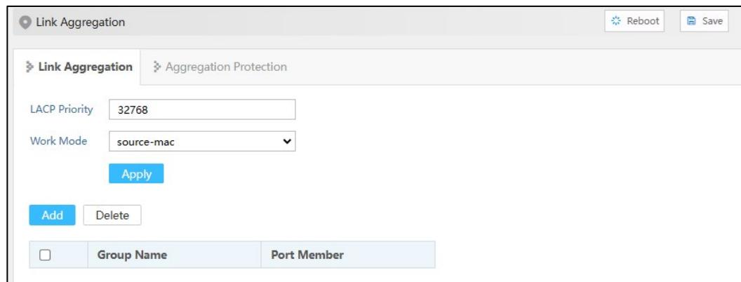
The screenshot shows a configuration interface for Link Aggregation. At the top, there are 'Reboot' and 'Save' buttons. Below that, there are two tabs: 'Link Aggregation' (selected) and 'Aggregation Protection'. Under 'Link Aggregation', there are fields for 'LACP Priority' (set to 32768) and 'Work Mode' (set to 'source-mac'). Below these are 'Apply', 'Add', and 'Delete' buttons. At the bottom, there are 'Group Name' and 'Port Member' fields.
