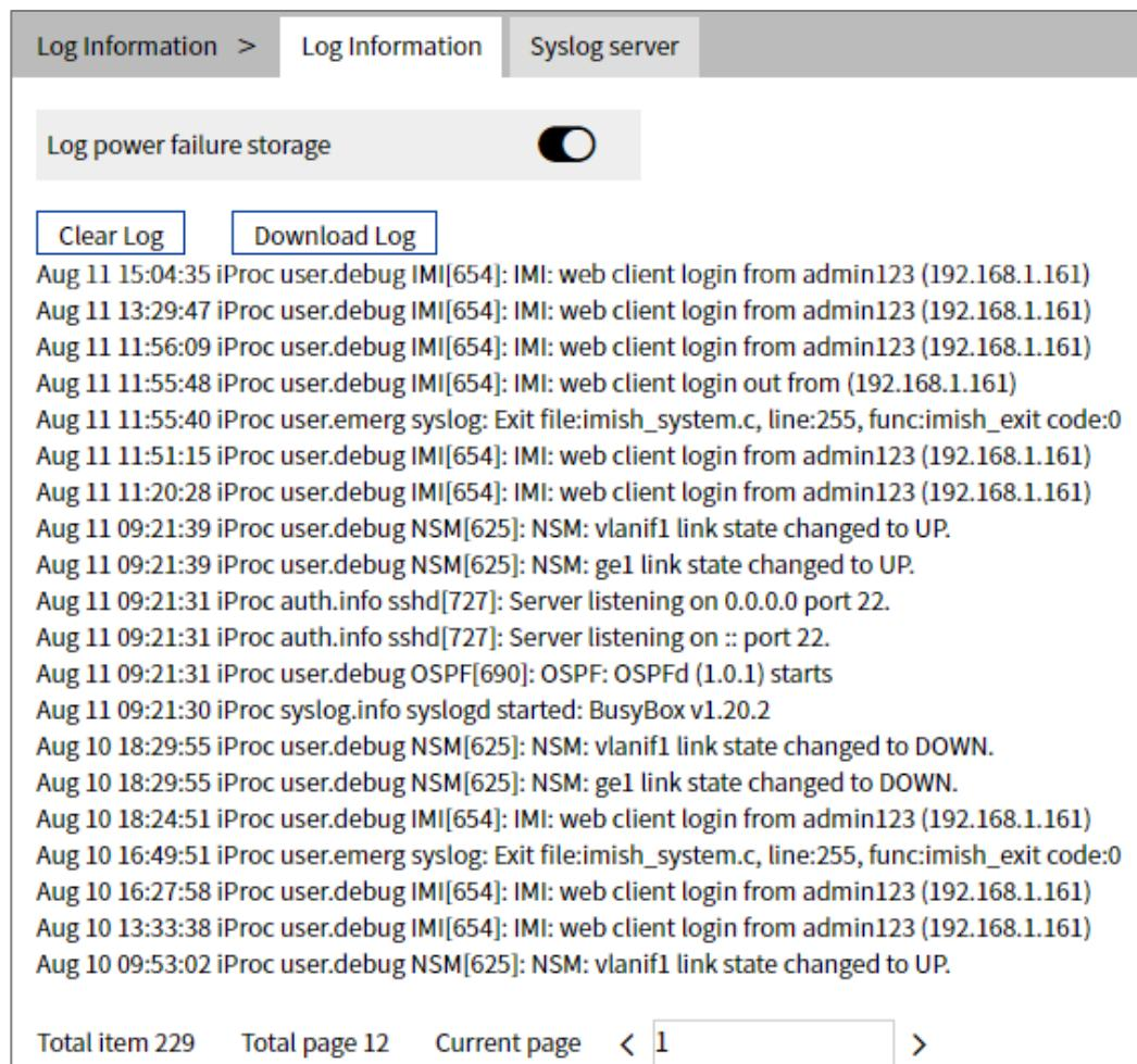
The screenshot shows the 'Log Information' page with the 'Log power failure storage' switch turned on. Below the switch are two buttons: 'Clear Log' and 'Download Log'. A list of log entries follows:
