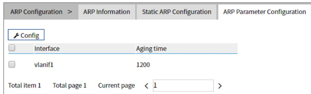
The main element configuration description of ARP Parameter Configuration interface:
