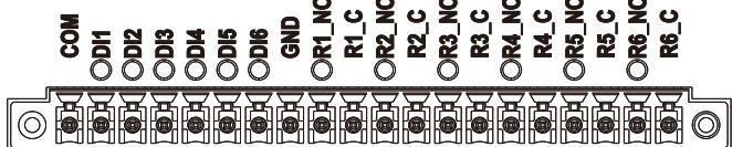
The device supports 6 digital inputs and 6 relay outputs channels, and adopts 20-pin 3.81mm pitch spring-loaded terminal block with screw latch. The definition of I/O pin is shown below.
